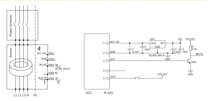
The detection module is sensitive to AC and DC currents and can be used for residual current detection of mode 2 or mode 3 charging equipment. The detection module detects AC and DC fault currents according to the IEC62752/IEC62955 standard requirements. In the case of an AC/DC fault current, PIN3 changes its state from a low level (GND) to a high-level state.
